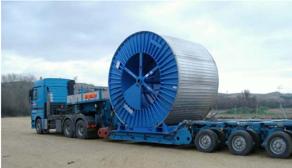
Figure 2.7: Cable Drum Transportation
